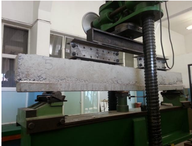
Figure 6: Failure pattern of test beam 5
