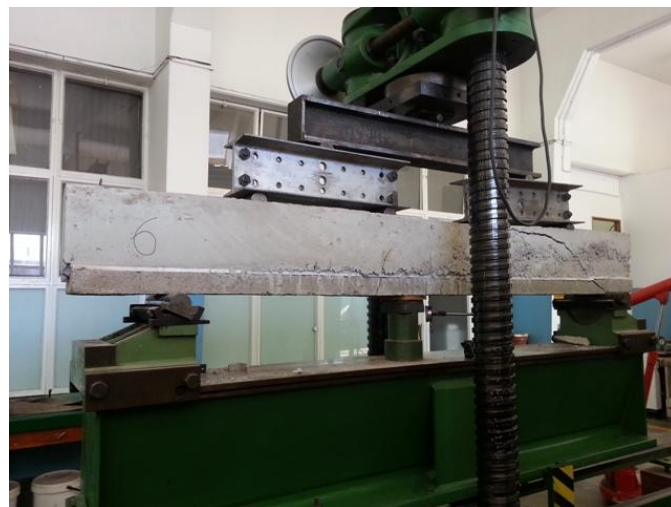
Figure 7: Failure pattern of test beam 6
