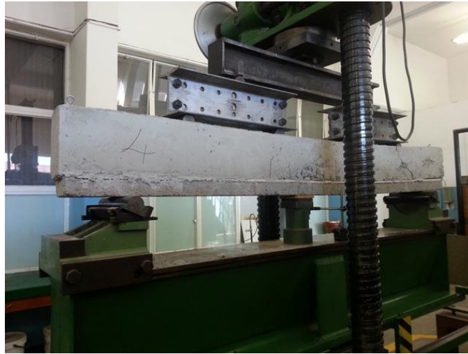
Figure 5: Failure pattern of test beam 4
