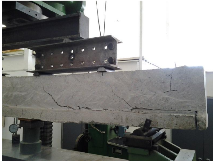
Figure 2: Failure pattern of test beam 1
